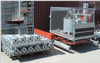
The material hoists ASClimber H-600 uses the same mast
